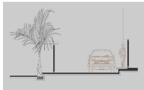
Figure 4 - entrance lower than street level .
